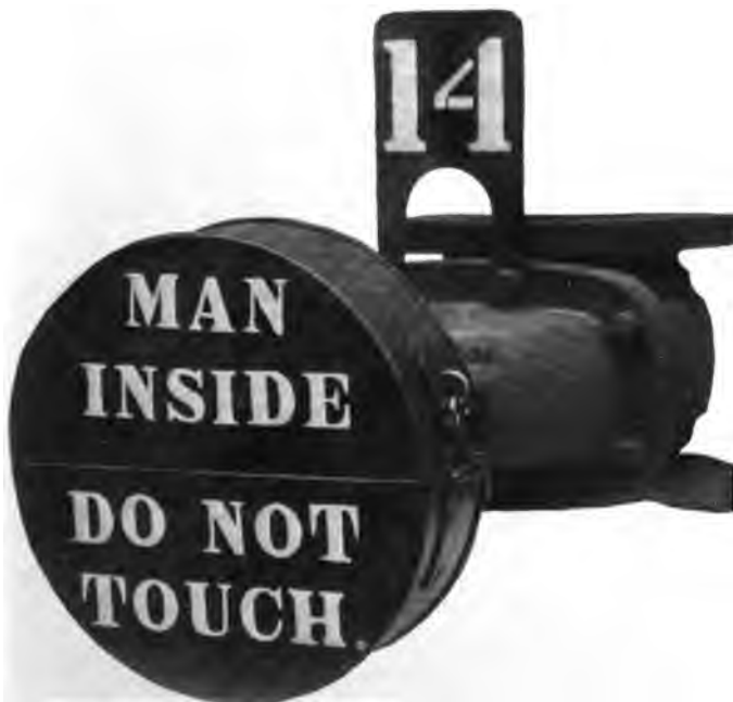
Fig. 3. Valve-Locking Device and Stencil for marking Main Steam Valve of Boiler.*
